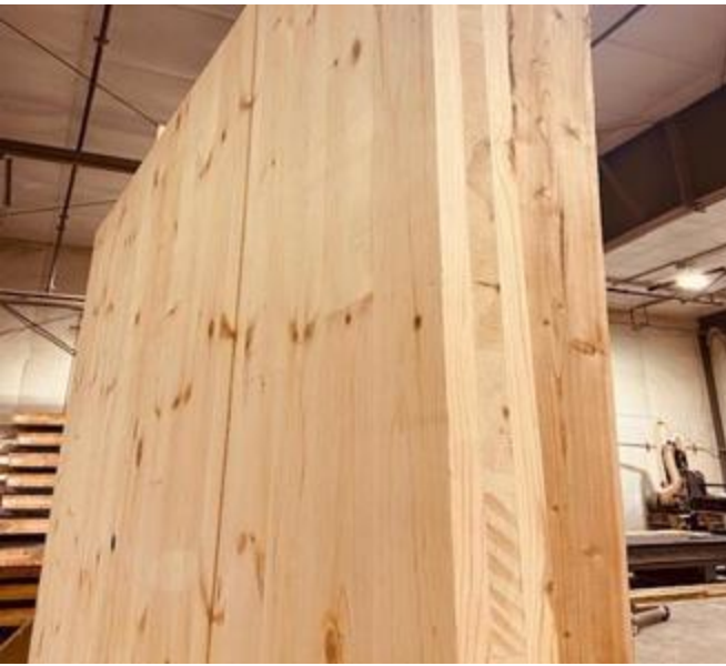
3PLY CLT WALL RED PINE PANEL
