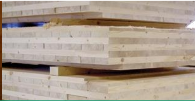
Cross-Laminated Timber (CLT)
